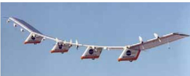
Centurion was a unique remotely piloted, solar-powered airplane craft designed to reach one of the goals of the ERAST program; to fly a payload of scientific data-gathering instruments for up to two hours at an ultra-high altitude of 100,000 feet.
