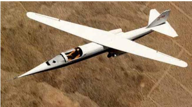
The Ames-Dryden-1 (AD-1) aircraft was designed to investigate the concept of an oblique (pivoting) wing. The wing could be rotated on its center pivot, so that it could be set at its most efficient angle for the speed at which the aircraft was flying.
