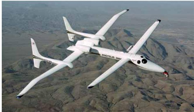
The Proteus is designed as a high-altitude, long-duration telecommunications relay platform with potential for use on atmospheric sampling and Earth-monitoring science missions. The Proteus is an "optionally piloted" aircraft ordinarily flown by two pilots in a pressurized cabin. The aircraft is designed to cruise at altitudes from 59,000 to 65,000+ feet for up to 18 hours.
