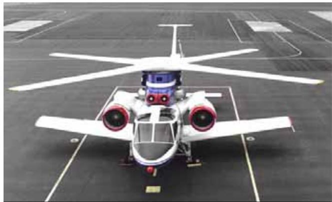
This unusual aircraft was conceived to provide an efficient combination of the vertical lift characteristic of conventional helicopters and the high cruise speed of fixed-wing aircraft. It consisted of a hybrid vehicle called the NASA Army Rotor Systems Research Aircraft (RSRA), which was equipped with advanced X-wing rotor systems.
