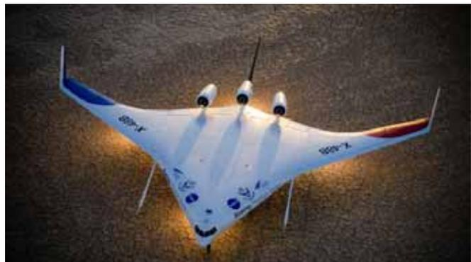
Boeing Phantom Works has partnered with NASA and the Air Force Research Laboratory to study the structural, aerodynamic and operational advantages of the Blended-Wing Body advanced aircraft concept, a cross between a conventional plane and a flying wing design. The Air Force has designated the prototype the X-48B based on its interest in the design's potential as a multi-role, long-range, high-capacity military transport aircraft.
